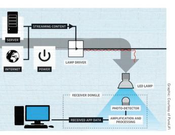
How It Works: An overhead lamp fitted with an LED with signal-processing techonolgy streams data embedded in its beam at ultra-high speeds to the photo-detector. A receiver dongle then converts the tiny changes in amplitude into an electrical signal, which is then converted back into a data stream and transmitted to a computer or mobile device.
