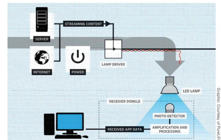
**How It Works:** An overhead lamp fitted with an LED with signal-processing technology streams data embedded in its beam at ultra-high speeds to the photo-detector. A receiver dongle then converts the tiny changes in amplitude into an electrical signal, which is then converted back into a data stream and transmitted to a computer or mobile device.
